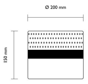
STEEL DROP, light magic in a steel case. For the new version of the e27 lamp, the precision steel light screen sits on an opaque metal base, separated by a thin band of black wood. The Traffic White model is an elegant study in black and white, while the black-on-black version emphasises the look of a technical element.
