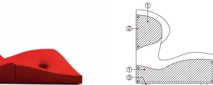
**ENG Structure** Injected flame-retardant foam ① over internal steel frame ②. Feet ③, screwed to the frame, in black polypropylene.
