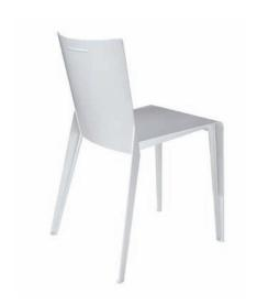
Alfa was born from the union of just two pieces: one is the back, which continues into the rear legs; the other is the seat that extends into the front legs. Both pieces are in "SMC" material, Polyester Resin, Fibre-glass re-inforced. Product certified UNI EN 1022/98 Stability Test, UNI EN 1728/00 Load and Resistance Test, UNI 8584/84 Resistance to Structural Fatigue.
